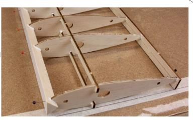
Glue and pin the triangle leading edge in place and allow to dry.
