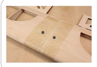
Using glass cloth (not supplied) run a section around the centre wing section and seal the wing. We recommend ZAP finishing resin. Repeat the process with the other wing. When dry cut out the holes for the servo leads.
