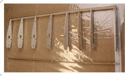
We recommend you build the wing on a building board so you can pin the trailing edge and wing ribs square to each other. It is imperative the wing is built square otherwise when you come to join the wing panels together it will be hard to align the wing panels. Before you pin the parts to the board glue the ribs to the trailing edge strip using a slow setting glue to allow working time.
