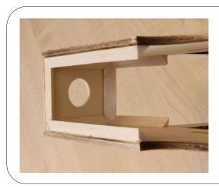
With the remaining triangle section re-enforce the firewall, undercarriage plate and top plate.
