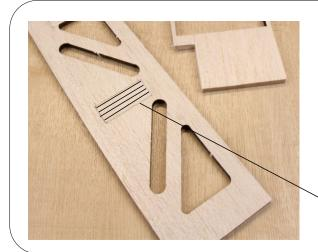
Using the outer section of the aileron that you kept from two steps ago, cut a section to fit the section shown, noting the grain direction, and glue in place.
