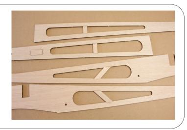
Glue in place the reinforcing strips on the fuselage sides and the top and bottom frames. Allow to dry and then sand.
