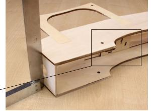
While gluing the two sides to the firewall make sure you keep the two frames parallel to each other.
