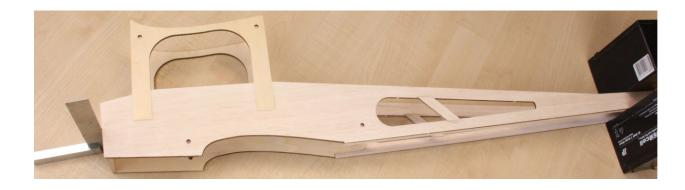
Insert the tailplane seat between the two fuselage frames and glue in place. It is very important when you glue this in place that you do not induce a banana shape to the fuselage.
