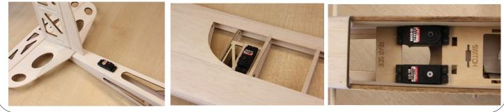
If you have chosen to put the rudder servo in the main servo tray please ensure you modify the servo tray before installation.
