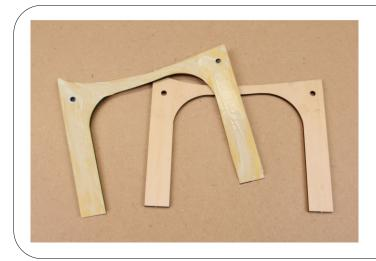
Prepare the four ply centre cabanes. Glue two of the cabanes together as shown in the image, when dry sand the edges but make sure you do not round the edges. Repeat the process for the other two pieces.
