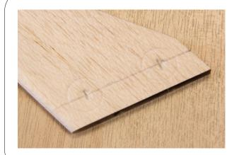
Mark a line 15mm in from either end of the wing strut. Then measure from the leading edge of the strut back 20mm along that line. Then measure again from the leading edge of the strut 60mm back. This is the position for the studs. When positions have been found press the stud down to mark the outer ring.
