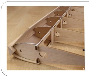
When the glue has set on the leading edge run slow setting glue on the ribs.
