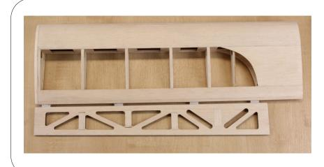
Please note this is for reference only for positioning of the hinges as this is normally done once the covering of your choice has been applied. We recommend four hinges per aileron. Hinges are not supplied in the kit.
