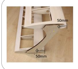
Position the wings on the plane and pin the strut to the top and bottom so the stud foremost is 50mm from the leading edge on both the top and the bottom. Repeat the same process on the other side. When you are happy with the positioning of the struts gently press the strut against the wing tip to make an impression on the wing tip so the press stud position can be located.
