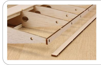
Carefully remove the trailing edge jig strip and sand the trailing edge to ensure it is flat.
