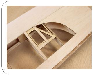
Using the wing rib capping strip make a box area around the servo tray as shown in the image.
