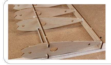
Make sure the wing ribs are sitting vertical to the build board. As mentioned before this is imperative for when it comes to joining the wing panels together.
