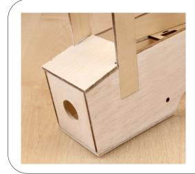
Glue in place the top plate ensuring it aligns with the centre cabanes.
