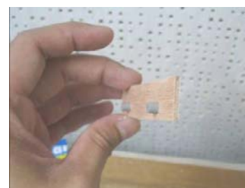
1. Install wing dowel D1 into SF4 and protrudes 6 mm. of the wood and then apply glue
