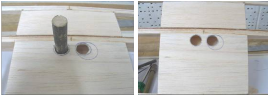
20. Drill holes for Y-connector exit and sand
