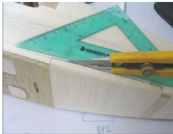
61. Use cutter to slitting battery hatch
