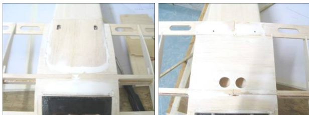
13. After the surface has dried, sand the area smooth
