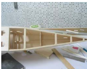
43. Make stringer by cutting P12 and assemble F 17 for tail wheel support
