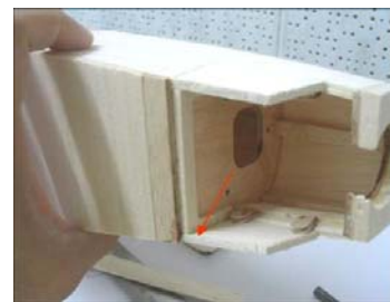
47. Place B 2 into position and trim B 3 (arrow point) to match with B 2
