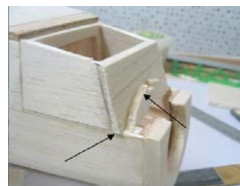
48. Assemble BP 1- B 7, arrow point show bevel line
