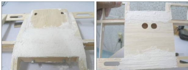
12. Fill any small gaps with balsa filler
