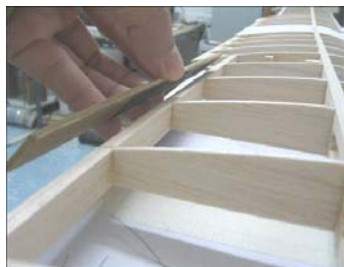
23. Use a bar sander to sand S 5 (be carefully the ribs)
