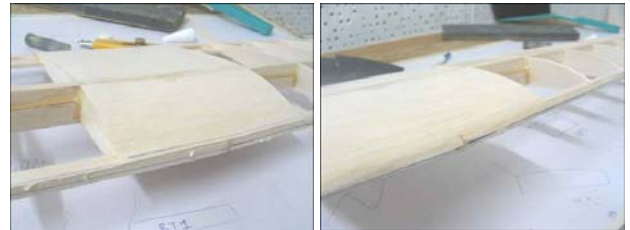
26. Mark the outline to round the leading edge of S 1
