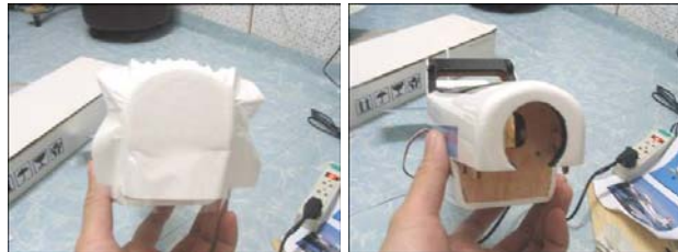
15. Iron F 0 and trim excess Monokote
