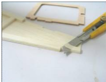
23. Before assemble F 8 trim P11 approximate 8 mm.
