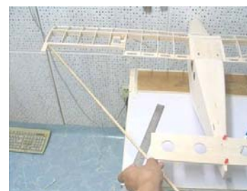
2. Mount the wing on the fuse, measure the distance from the aileron bay to the TE corner of the stab. Adjust the stab until both distances are equal. When satisfied with the fit, glue stab to the fuse
