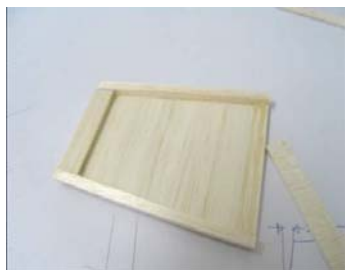
62. Assemble BT1 as shown; cut the 10x78x3 mm balsa strip for battery hatch stop
