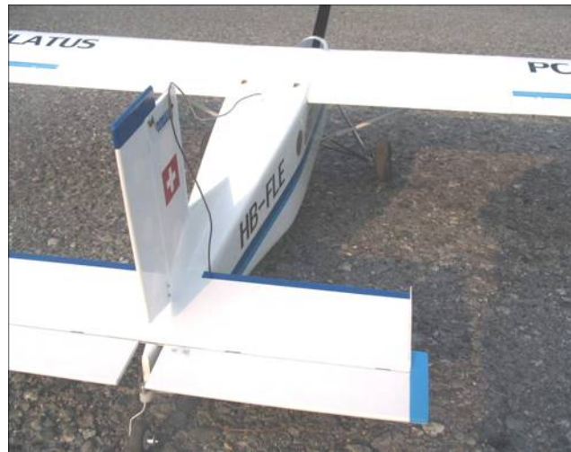
Prototype using HBT brushless motor A22/15 1000 Kv motor weight 69 grams 9x5 propeller
