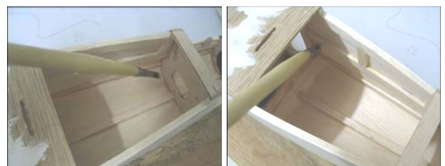
15. Apply Epoxy inside of fuselage as shown
