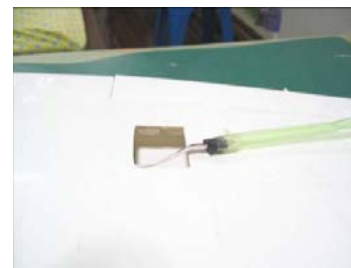
22. Tape Y-connector with straw to guide the wire through the wing and out the hole
