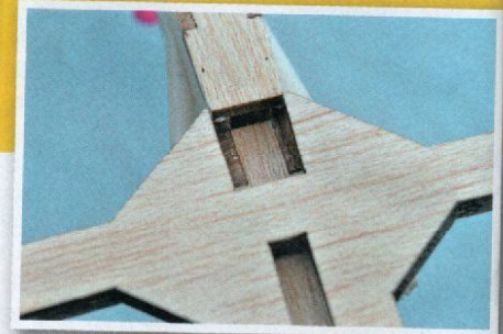
A bit of sanding was needed to make the tailplane slot fit the fuselage.
