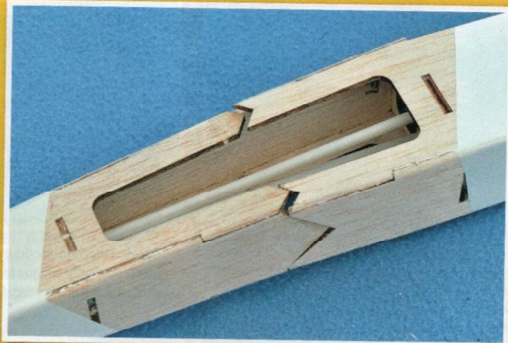
Blast! My mistake. I used cyano for the joint and it couldn't stand the poor arrival on Mother Earth. It has since been repaired and reinforced, a simple job.
