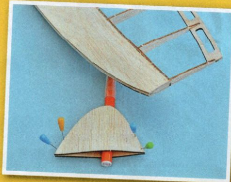
Pre-curving the wingtips before gluing gives a tidier top surface.
