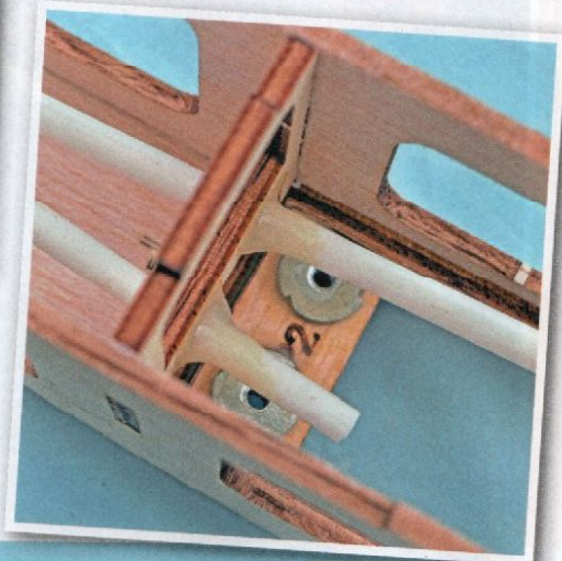
When fitted the pushrod outers form a curve through the fuselage side which makes the supplied fibreglass pushrods 'stick'. Replace with 1.0 to 1.2mm dia. piano wire and the problem is solved.
