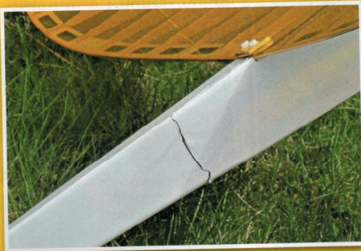
Oh dear! A difficult landing shows up a fuselage weakness.
