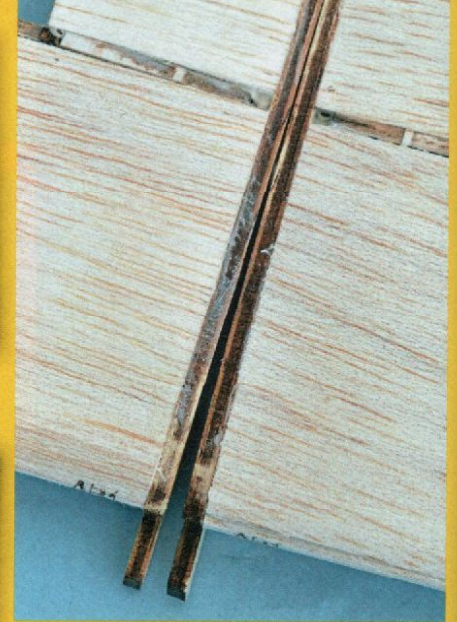
Oops! I didn't allow for the rib tilt needed for the dihedral break and this is the result. A bit of judicious sawing and an epoxied ply filler sorted it.
